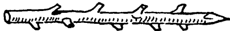
Meat Loaf Stick : The barbs or branches keep the meat loaf from turning. Make 1/2" in diameter, 12" long.
